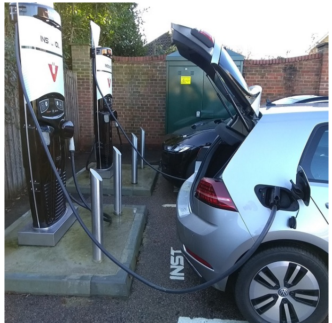
Figure 8: Two vehicles charging simultaneously. With the eavesdropper between the two vehicles 42.5% of messages were received successfully, including the NMK key establishment for both vehicles.
