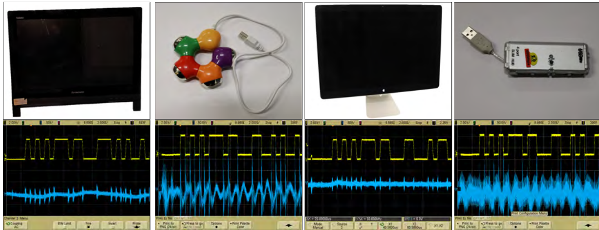
Figure 7: Top row: four tested USB hubs found to contain power line crosstalk leakage. Bottom row: Corresponding leakage waveform, yellow (top) trace shows the USB traffic and blue (bottom) trace shows the power line crosstalk leakage measured from an adjacent downstream USB port. Notice the correlation between the sharp spikes in the leakage trace and the USB traffic. The waveforms were captured using an Agilent MSO6104A oscilloscope (1GHz, 4Gps) and two Agilent 10073C 500MHz passive probes.
