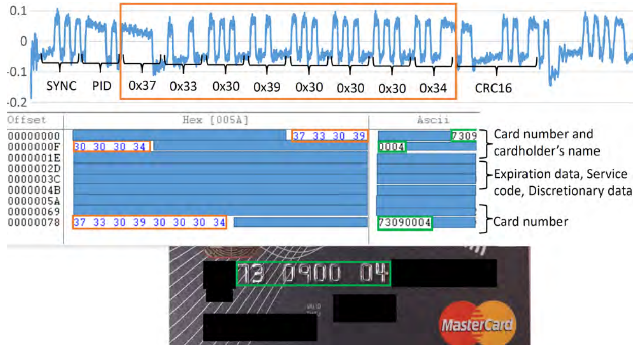
Figure 17: Extracted credit card data using data line crosstalk leakage. (top) Observed data line crosstalk leakage trace segment. Part of the credit card number is visible in hexadecimal encoding (marked in orange box). (middle) hexadecimal to ascii conversion of the extracted data. Part of the credit card number is visible in ascii form (green). (bottom) picture of the credit card used. Notice the correct extraction of the credit card number. In order to protect owner's privacy we have hidden all other card details.
