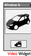
Figure 3: A photo capturing application presents a video camera widget, instead of a camera widget, to trick the user into also granting access to the microphone. The windowing display context surrounding the widget shows a camera preview for photo capturing.
