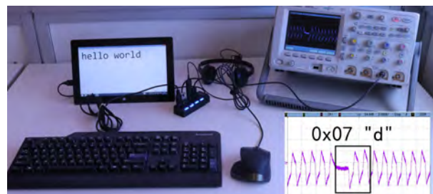
Figure 15: Extracting keyboard presses using data line crosstalk leakage. The scan code 0x07 corresponding to the letter d is clearly visible in the leakage trace.
