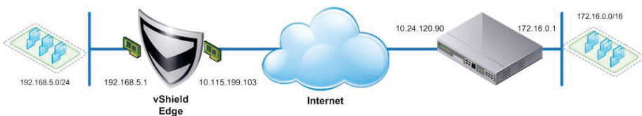
Figure 58. Point-to-Point IPsec VPN Connection between vShield Edge and Physical Gateway VPN
