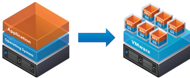
Figure 2: Virtualization groups App/OS pairs into virtual machines.
